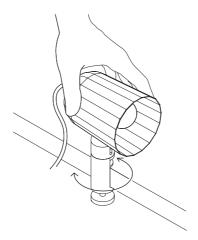
Loosen the head adjustment grip to adjust the angle of the head.
